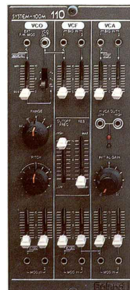
VCO/VCF/VCA section in Roland's System 110m
